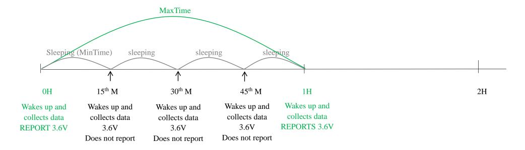
Example#3 based on MinTime = 15 Minutes, MaxTime= 1 Hour, Reportable Change i.e. BatteryVoltageChange= 0.1V.
